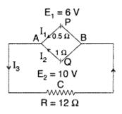
(ii) Calculate the value of the resistance R in the circuit shown in the figure so that the current in the circuit is 0.2 A. What would be the potential difference between points B and E?
