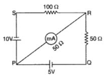
11. Use Kirchhoff's rules to determine the value of the current  $I_1$  flowing in the circuit shown in the figure.
