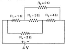
6. In the given circuit, assuming point A to be at zero potential, use Kirchhoff's rules to determine the potential A at point B.
